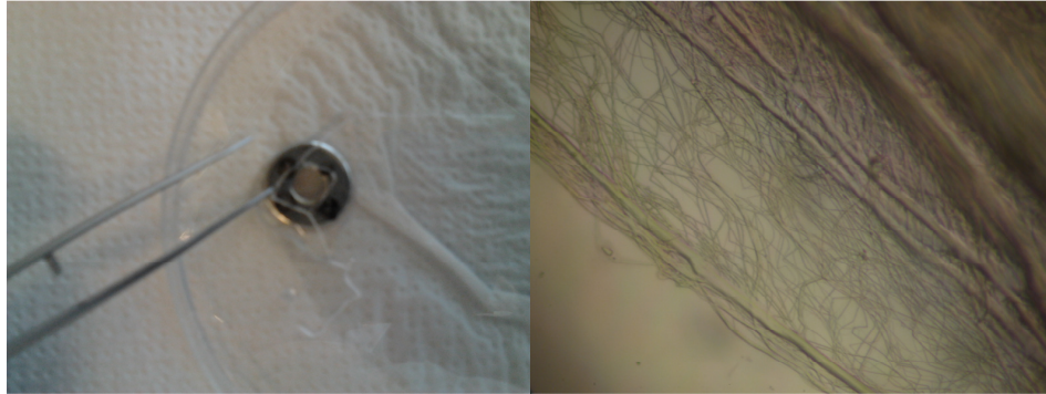
Figure 17: Left: Fiber bundle is opened up under fluid by tweezers to expose individual collagen fibers. Right: Individual collagen fibers.
