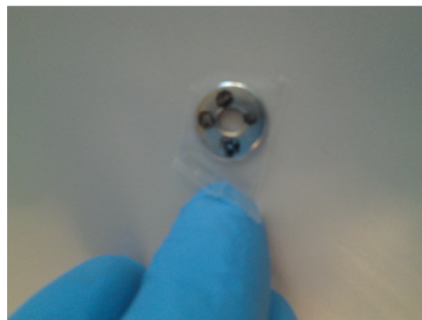
Figure 15: Mica on a metal support is cleaved by removing scotch tape.
